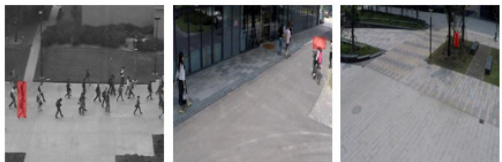
Figure 9. Several imperfect cases of anomaly localization affected by Mask R-CNN detector. Left: Too large bounding box; Middle: Too small box; Right: Wrong object. Best viewed in color.
