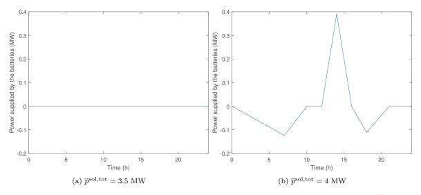
Figure 9: Evolution of total active power supplied by batteries for  $c_{\text{bat}} = 2 \text{ MW}^{-1}$
