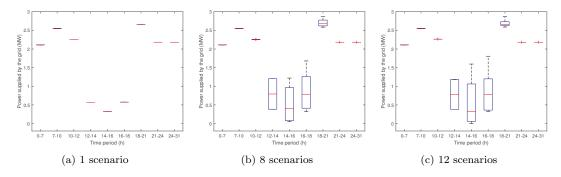
Figure 8: Empirical distribution of active power injections at bus 0 over time
