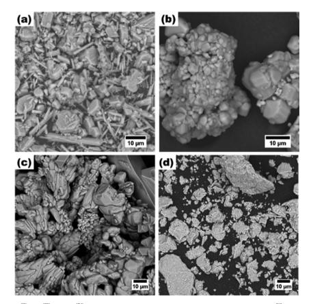
Fig. 4. SEM micrographs of the (a) V<sup>(II)</sup>, (b) V<sup>(III)</sup> and (c) V<sup>(IV)</sup> precipitates obtained after 4 days of the 30 °C aging process, and (d) V<sup>(V)</sup> precipitates obtained after 30 days at the 60 °C.
