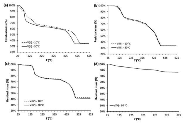
Fig. 6. Thermogravimetric analysis of the (a) V<sup>(II)</sup>, (b) V<sup>(III)</sup> and (c) V<sup>(IV)</sup> precipitates obtained after 4 days aging process at 10 or 30 °C and (d) of the V<sup>(V)</sup> precipitates obtained after 30 days aging process at 60 °C.
