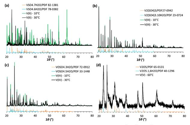
Fig. 5. X-ray diffraction patterns of the precipitated phases obtained after 4 days at 30 °C and 10 °C from (a) V<sup>(II)</sup>, (b) V<sup>(III)</sup> and (c) V<sup>(IV)</sup> solutions; (d) after 30 days at 60 °C for V<sup>(V)</sup>.
