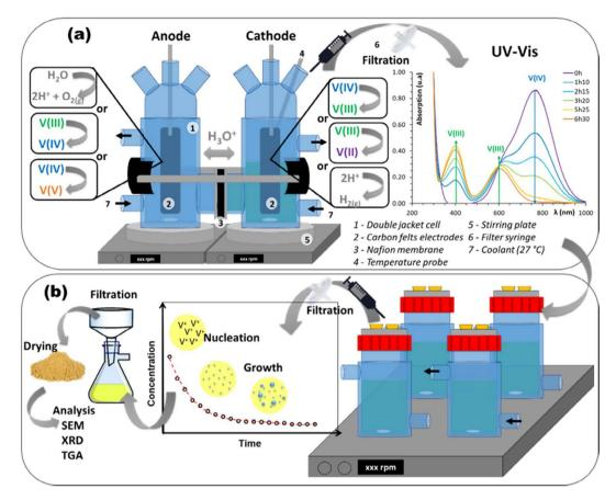
**Fig. 1.** Schematic representation of the overall procedure of the preparation of the four valences of vanadium sulfate salts. (a) Electrolytic preparation in a two-compartments electrolytic cell coupled with spectroscopic analysis. (b) Aging/precipitation of the vanadium supersaturated solutions in stirred and thermoregulated vessels and filtration and drying of the precipitates.
