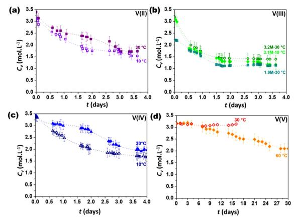
**Fig. 3.** Temporal evolution of the concentrations of the four valences of vanadium in supersaturated electrolytes during their aging/precipitation process at constant stirring rate (400 rpm), two different constant temperature (10 °C and 30 °C for V<sup>(II)</sup>, V<sup>(III)</sup> and V<sup>(IV)</sup> and 30 °C and 60 °C for V<sup>(V)</sup>) and two vanadium initial concentration for V<sup>(III)</sup>.
