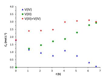
**Fig. 2.** Evolution of the concentrations of  $V^{(IV)}(\blacktriangle)$ ,  $V^{(III)}(\bullet)$  and total vanadium ( $\blacklozenge$ ) during an electrolysis at T = 27 °C by applying 1 A for 6.7 h in 50 mL of a stirred (400 rpm) suspension containing 5 mol.L<sup>-1</sup> H<sub>2</sub>SO<sub>4</sub> and an initial total quantity of  $V^{(IV)}$  of 3.15 mol.L<sup>-1</sup>.
