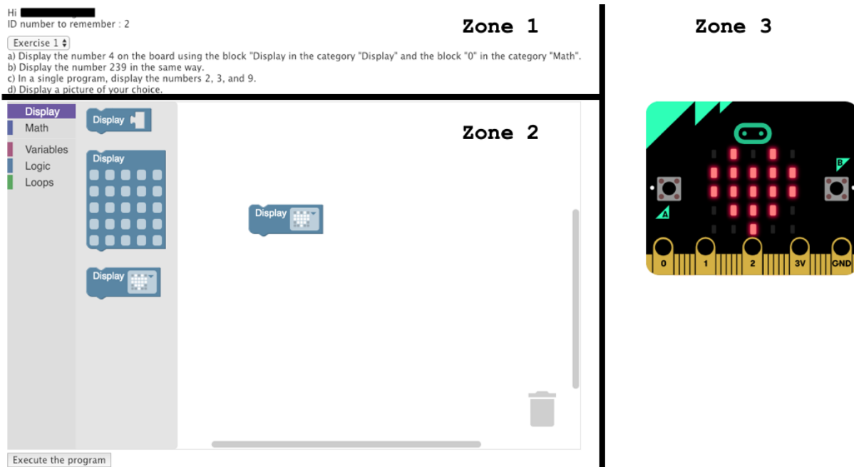
Figure 2: The block-based Web interface for programming the simulation of the micro:bit.
