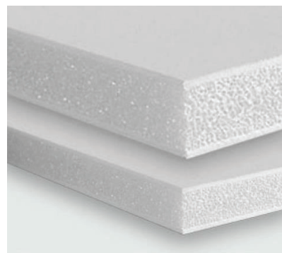
Figure 9. Example of foamboard sheets, showing the sandwich structure with inner polystyrene foam core and two outer layers of paper (source: www.indiamart.com).
