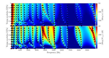
Figure 2. Waterfall representation of field displacement responses (at the top) and of radiation power (at the bottom) from a parametric study where the pad Young modulus,  $E_p$  changes from 0 (no contact between beams) to 1 GPa (10 times stiffer than strong caoutchouc). Lines represent responses and are classified as bending bending response, (black triangle), pure compression response (green dot) or a combination of both movements, called hybrid responses (red square).
