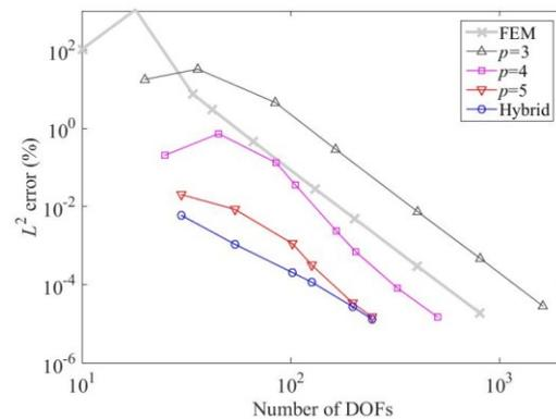
**Figure 1.** Convergence curves with mesh refinement for classical FEM, the PUFEM with polynomial enrichment of different orders  $p$  and hybrid enrichment combining progressive waves and cubic polynomials ( $f=1000$  Hz).
