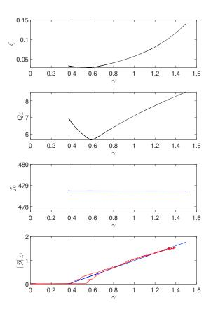
Figure 1. Results from continuation with constraints. Evolution of  $\zeta$ ,  $Q_L$ ,  $f_0$  and  $\|\tilde{p}\|_{L^2}$  with respect to the dimensionless mouth pressure  $\gamma$ . In red is the evolution of  $\|\tilde{p}\|_{L^2}$ with respect of  $\gamma$  measured on trumpet player during a slow crescendo-decrescendo maneuver.
