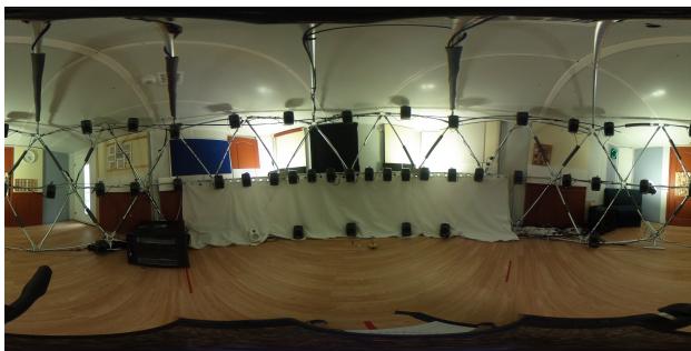
Figure 5. Panoramic photograph of the 42.1 loudspeaker setup used in the audiobooth at University of Surrey.
