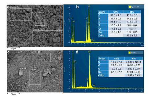
**Figure 4.** (**a**,**c**) Backscattered SEM image and (**b**,**d**) corresponding EDX spectra of the as-synthesized PANI-based materials: (**a**,**b**) PANI-Ru-nc, and (**c**,**d**) PANI-Ru-c. Please: Read "Spectre" as "Spectra".
