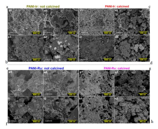
**Figure 2.** (**a**,**c**,**e**,**g**) Normal scanning electron microscopy (SEM), and (**b**,**d**,**f**,**h**) the corresponding backscattered images of the as-synthesized PANI-based materials: (**a**,**b**) PANI-Ir-nc, (**c**,**d**) PANI-Ir-c, (**e**,**f**) PANI-Ru-nc, and (**g**,**h**) PANI-Ru-c.
