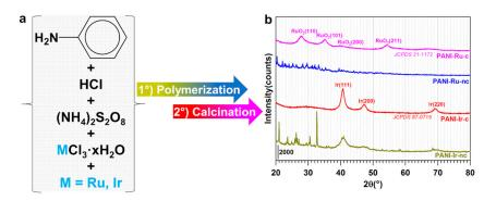
**Figure 1.** (a) Sketch of the developed methodology leading to uncalcined materials (polyaniline (PANI)-Ir-nc, and PANI-Ru-nc), and calcined ones (PANI-Ir-c, and PANI-Ru-c); (b) XRD of the prepared materials.
