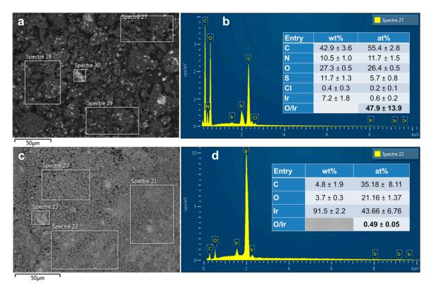
**Figure 3.** (*a*,**c**) Backscattered SEM image and (*b*,*d*) corresponding energy-dispersive X-ray spectroscopy (EDX) spectra of the as-synthesized PANI-based materials: (*a*,*b*) PANI-Ir-nc, and (*c*,*d*) PANI-Ir-c. Please: Read "Spectre" as "Spectra".
