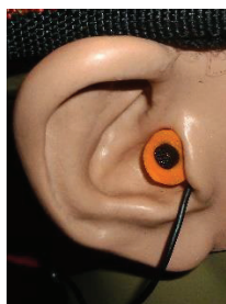
Figure 1: Microphone at the entrance of the ear canal
