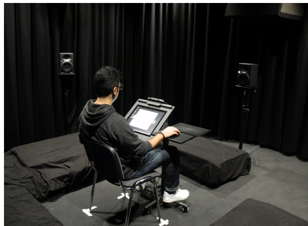
Figure 2. The experimental setup in AuraLab: the subject was seated in the central listening spot. The stimuli were played back through five satellite loudspeakers and two subwoofers.
