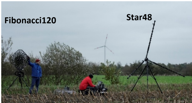
Figure 6: Picture of a full measurement setup consisting of both arrays, data acquisition system and computer
