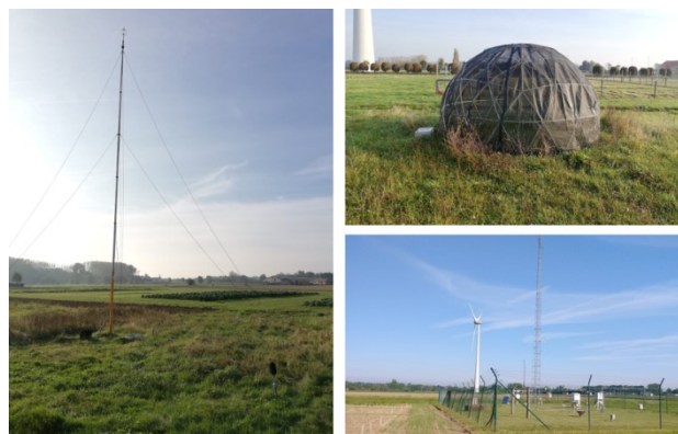
Figure 3. Field measurement set up: sonic anemometer at 10 m height (left), wind-shielding dome covering the microphone (right, up) and the meteorological station (right, down)
