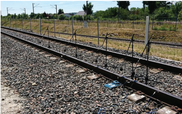
Figure 6. Microphones close to the rail for the calibration of rail acoustic impedances
