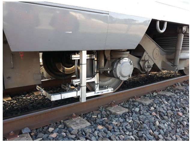
Figure 3. Supporting structure for near-field microphones (wheel and rail)
