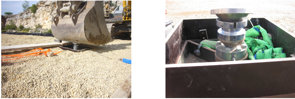
Figure 3. Experimental loading system: 34 tonne excavator (a) acting on a hemi-spherical head linked to the force sensor (b).
