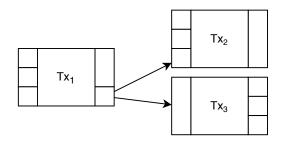
Figure 2:  $Tx_2$  and  $Tx_3$  both use the same funds (the second output of  $Tx_1$ ). This is considered double-spending and is not allowed. Hence,  $Tx_2$  and  $Tx_3$  are in conflict and a miner cannot include both of them in her block.
