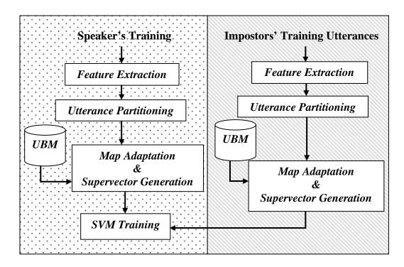
Fig. 1 Training of GMM-SVM classifier with partitioning of training utterance (UP) approach.
