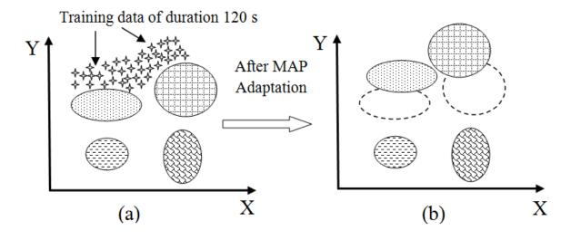
Fig. 4 Preparation of the training GMM supervector using MAP adaptation from UBM. Here, 4 (a) indicates the condition before MAP adaptation and 4 (b) indicates the condition after MAP adaptation.
