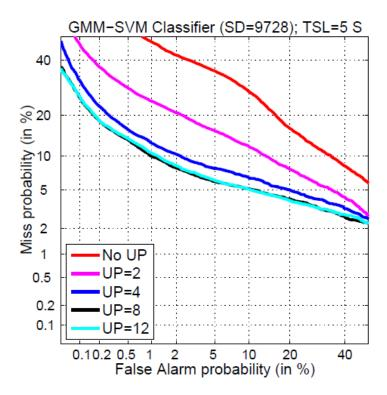
Fig. 8 Effect of partitioning of training utterance (UP) on the performance of GMM-SVM classifier with GMM supervector of dimension (SD) 9728 for recognition of test segments of short duration (5 s). Here, TSL=test segment length.
