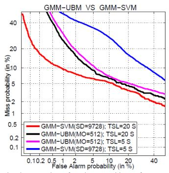
Fig. 2 DET curves showing the comparison of speaker recognition performances between GMM-UBM classifier of model order 512 and GMM-SVM classifier with GMM supervector of dimension 9728 for recognition of test speech segments of long and short durations.
