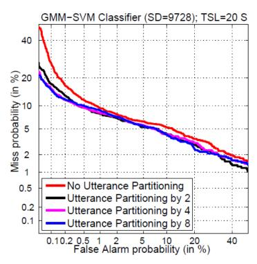
Fig.7 Effect of partitioning of training utterance (UP) on the performance of GMM-SVM classifier with GMM supervector of dimension (SD) 9728 for recognition of test segments of long duration (20 s). Here, TSL=test segment length.
