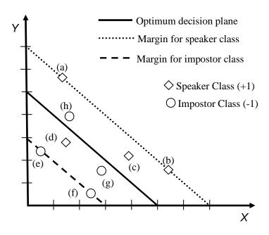
Fig.16 Different positions possible for the support vectors of the SVM classifier with a soft margin decision boundary.
