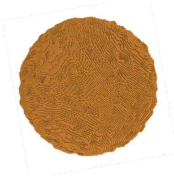
FIGURE 2. Nanosphere with rough surfaces designed for atomistic simulations using spherical harmonics.
