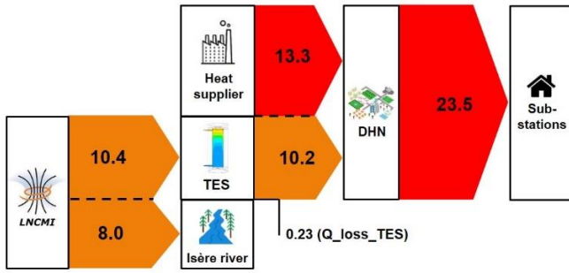
Figure 10a. Sankey diagram (energy flows in GWh/year) for the optimized operation of the WHRS with a source-oriented, energy-based optimal design (i.e. waste heat at 85 °C, and no heat pump). This design is also supported by the exergy-based optimization.
