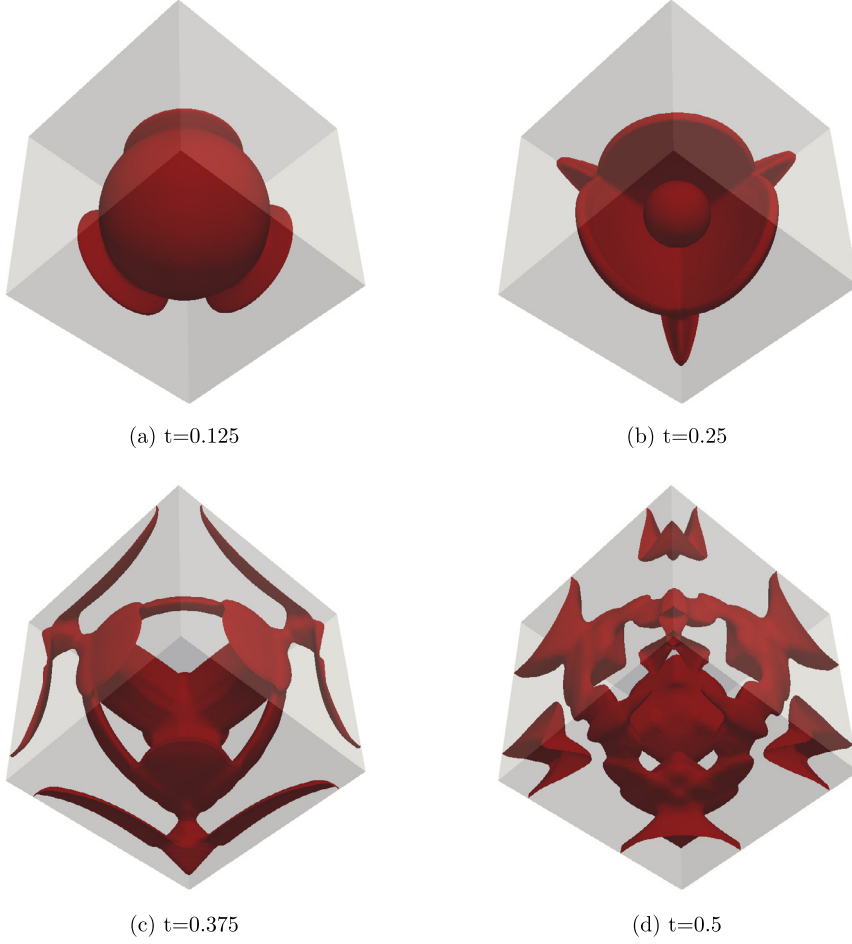
Fig. 11. Instantaneous density isosurface of \rho = 1.8 in the 3D enclosed box.
