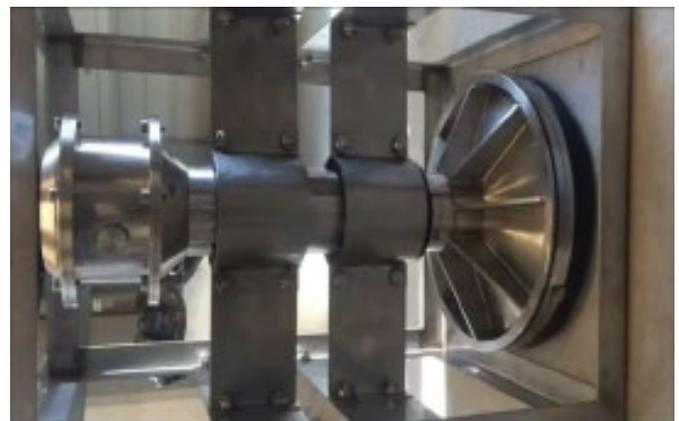
**Figure 9.** Photography of the ultra-wide band transducer.
