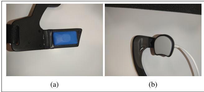
Figure 2: Two bone conduction transducers evaluated in this paper: (a) B1, prototype from the ELNO company, (b) B2, commercial sports headset.
