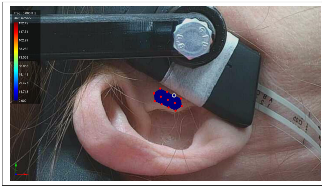
Figure 3: Photograph of the SLDV measurement setup. 15 measure points (in red) are placed on the subject's tragus.
