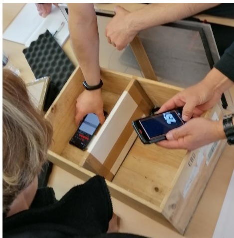
Figure 9: Highlighting of the acoustic transmission through a wall based on a scale model of room.
