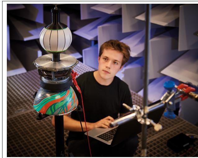
Figure 4. Radialstrahler prototype ready to be measured in the anechoic room.
