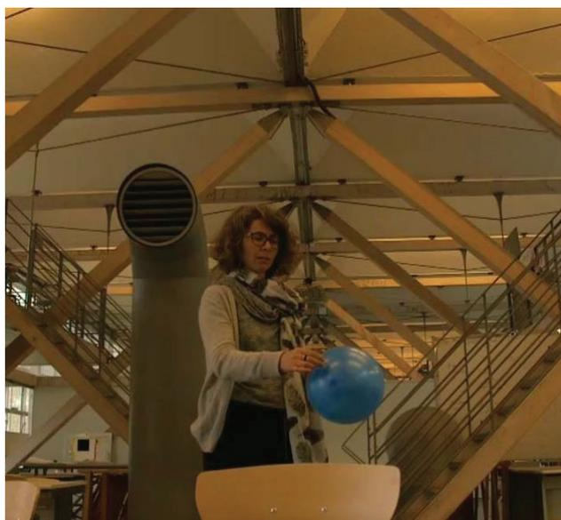
Figure 6. Reverberation balloon test of, ENSA Lyon, Laboratoire des Ambiances 2016
