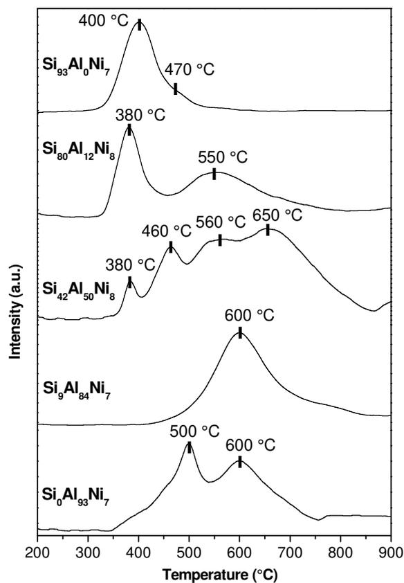
**Figure 7:** H<sub>2</sub>-TPR profiles of Si<sub>x</sub>Al<sub>y</sub>Ni<sub>z</sub> samples.
