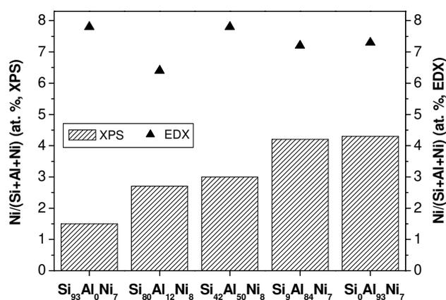
**Figure 6:** XPS (left axis, striped bars) and EDX (right axis, filled triangles) Ni/(Ni + Si + Al) atomic ratios for catalysts as a function of the Al<sub>2</sub>O<sub>3</sub> weight loading.
