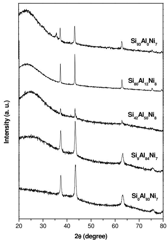
**Figure 3:** Powder XRD patterns of  $\text{Si}_x\text{Al}_y\text{Ni}_z$  samples.
