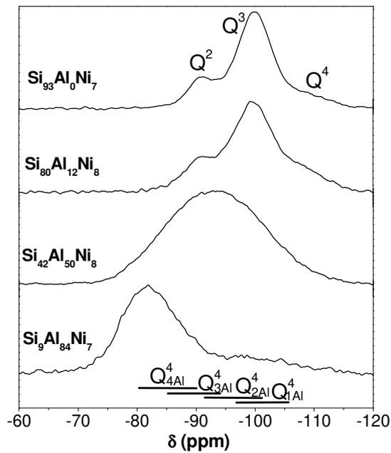
**Figure 1:**  $^{29}\text{Si}$  CP-MAS NMR spectra of  $\text{Si}_x\text{Al}_y\text{Ni}_z$  samples.
