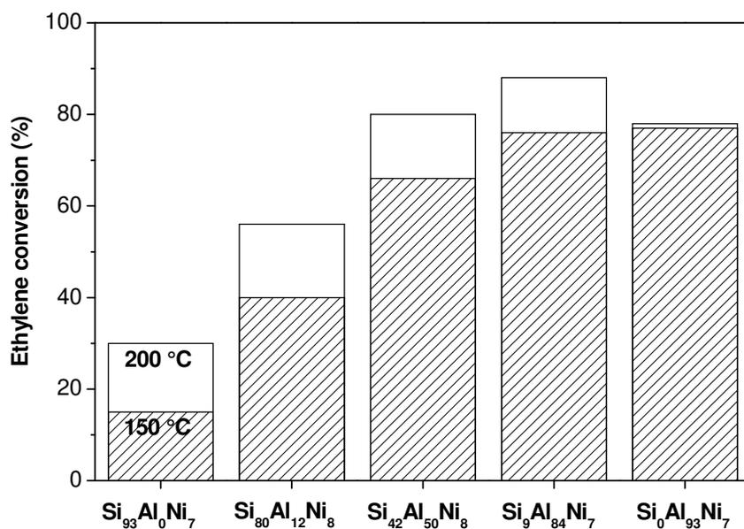
**Figure 8:** Ethylene conversion at 150 °C (striped bars) and 200 °C (empty bars) over the Si<sub>x</sub>Al<sub>y</sub>Ni<sub>z</sub> catalysts.
