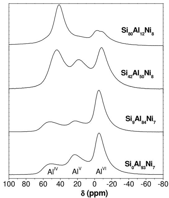
**Figure 2:**  $^{27}\text{Al}$  MAS NMR spectra of  $\text{Si}_x\text{Al}_y\text{Ni}_z$  samples.
