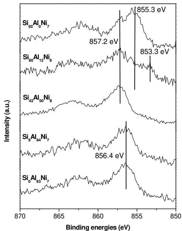
**Figure 5:** Ni<sub>2p3/2</sub> XPS spectra of Si<sub>x</sub>Al<sub>y</sub>Ni<sub>z</sub> samples.
