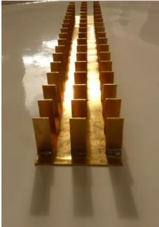
Fig. 3: Metamaterial structure designed at 1 GHz
