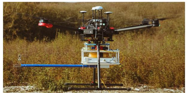
Fig. 5: Measurement system aboard the UAV
