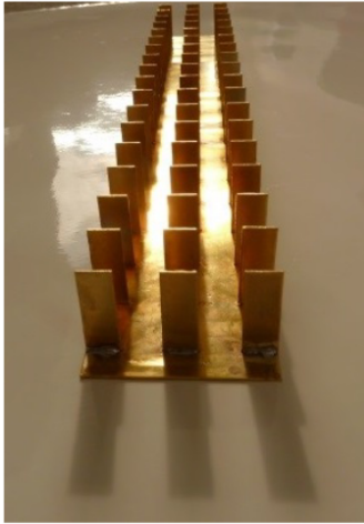
Fig. 3: Metamaterial structure designed at 1 GHz
