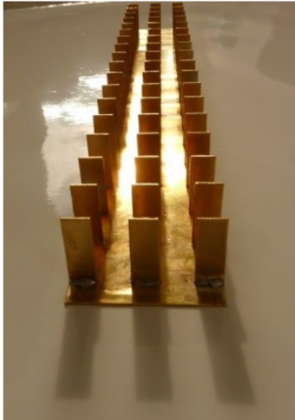
Fig. 3: Metamaterial structure designed at 1 GHz
