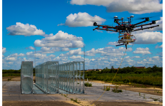
Fig. 1: 3D metamaterial used in HF band and the near field measurement system embedded aboard a UAV
