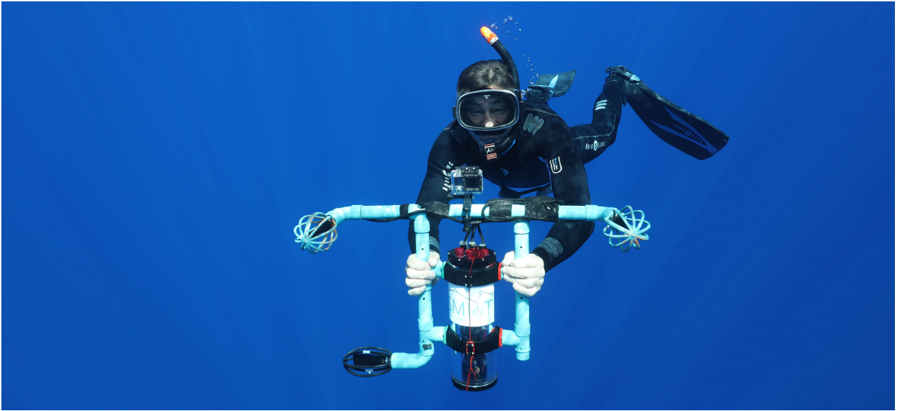
Figure 4. F. Sarano holding the antenna, version 2018, designed and built by H. Glotin (Image: F. Guerin). The hydrophones are three Cetacean Research, at the top two CR55 spaced by 60 cm, at the bottom a CR305.
