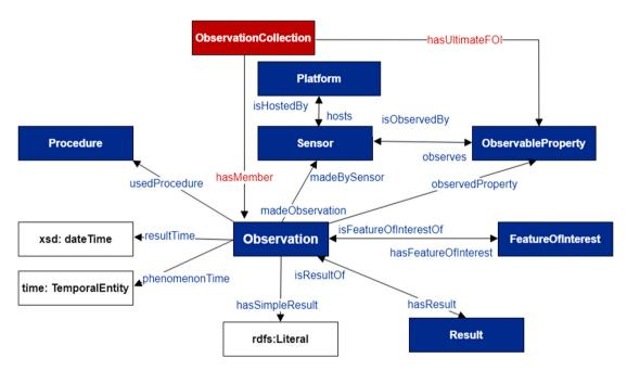
Fig. 3. Extensions to the semantic sensor network ontology (Cox and Little, 2020).
