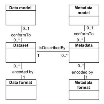
Fig. 1. Relationships among dataset, data model, data format, metadata model and metadata format.
