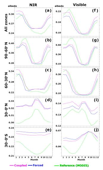
**Figure 5.** Monthly climatological time series of global and zonal mean albedo. The left column shows the NIR band ( $\mathbf{a}$  – global average;  $\mathbf{b}$ – $\mathbf{e}$  – zonal average for each 30° in latitude), while the right column ( $\mathbf{f}$ – $\mathbf{j}$ ) shows the visible band (the vertical arrangement is the same as that for NIR).
