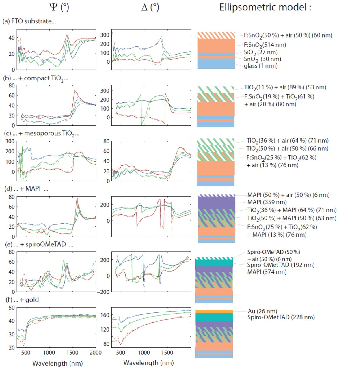
Figure 2 : Left and middle columns : measured (full lines) and fitted (dotted lines) ellipsometric curves at each successive step of sample deposition, at incidence angles  $50^{\circ}$  (blue),  $60^{\circ}$  (green) and  $70^{\circ}$  (red). Right column : model structure obtained by fitting the ellipsometric data (EMA layers are represented by hatches). This structure will define the 1D model used in the following of the paper.
