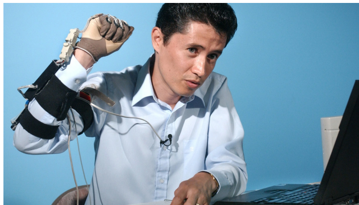
Figure 8: Prototype sign language sensor gloves (Erard 2017)
