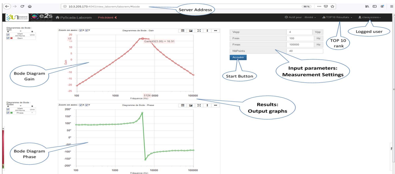
Figure 6. The student interface of Laborem. Bode diagram of a second order band pass active filter.
