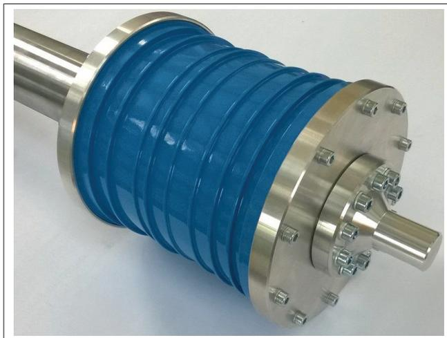
**Figure 3.** Examined electric motor (an external rotor motor with air gap winding).
