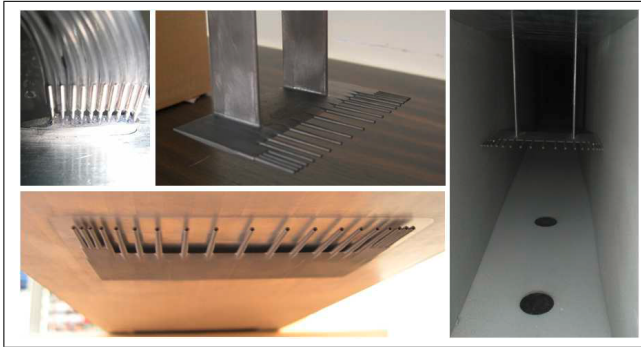
Figure 8. Pictures of the Pitot comb.
