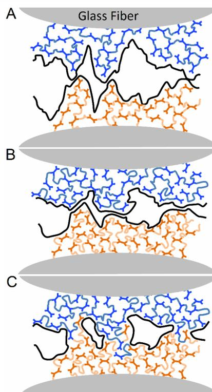
**Figure 1.** Schematic view showing the mechanisms expected to promote significant adhesion when two epoxy vitrimer composite plates are put in contact under a load  $P$  at high temperature  $T$ . **A**→**B** Exchange reactions within the vitrimer network enable the matrix to flow thus increasing surface conformity and fostering the contact between top and bottom adherands; **B**→**C** Upon contact, exchange reactions between top and bottom adherands occur, creating bonds at the interface.
