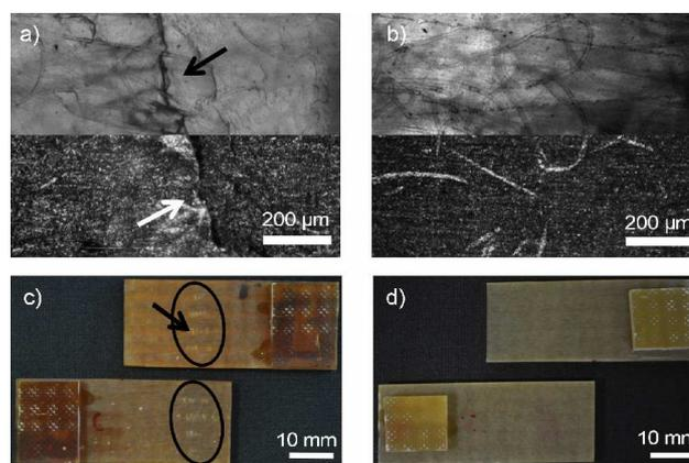
**Figure 6.** Microscopic observations by transmission (top) and reflection (bottom) of the surface of an epoxy vitrimer 2:1-Zn (a) and a reference 2:2 (b) lapjoint specimens after rupture (1<sup>st</sup> sticking, 160°C, 1h30, 1.7 MPa). Visual aspect of the same samples showing cracks on the epoxy vitrimer (c) and an essentially flat surface for the reference (d).
