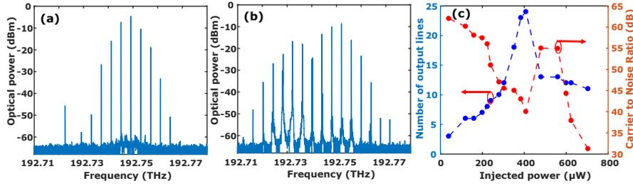
Fig. 2. (a), (b) optical spectra of VCSEL output for fixed comb spacing to  $\Omega = 4 \text{ GHz}$ . (a) and (b) are obtained for  $P_{inj} = 432.8 \mu\text{W}$  and detuning  $\Delta\nu = -2.6 \text{ GHz}$  and  $\Delta\nu = -5.4 \text{ GHz}$ , respectively. (c) OFC performance analysis for fixed  $\Delta\nu = -0.9 \text{ GHz}$ .
