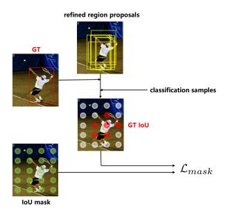
Fig. 3. The generation of supervision information and the training phase of Light-weight IoU-Mask branch. As a result, red points in ground-truth IoU map denote the ground-truth of training samples, while white points denote the irrelevant samples.
