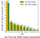
Fig. 7. The changes in the IoU distribution of region proposals with and without IoU mask. Here, (a) and (b) describe the changes in the IoU distribution of the top 300 region proposals and the top 1000 region proposals, respectively. Both (a) and (b) verify that IoU mask can refine the classification scores of region proposals and prevent the high-quality region proposals from being removed in NMS.
