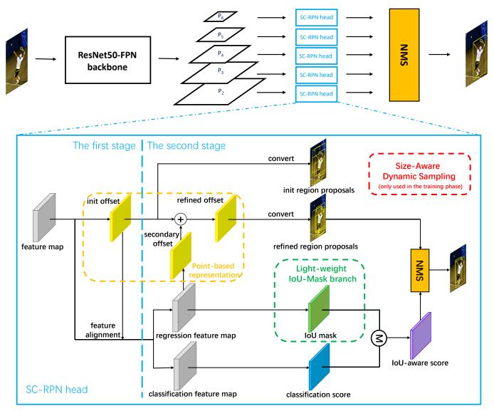
Fig. 1. The overall pipeline of SC-RPN. IoU mask is predicted by the Light-weight IoU-Mask branch and region proposals are described by the point-based representation. In addition, Size-Aware Dynamic Sampling (SADS) is used for generating the training samples and calculating the losses, which is only used in the training phase.
