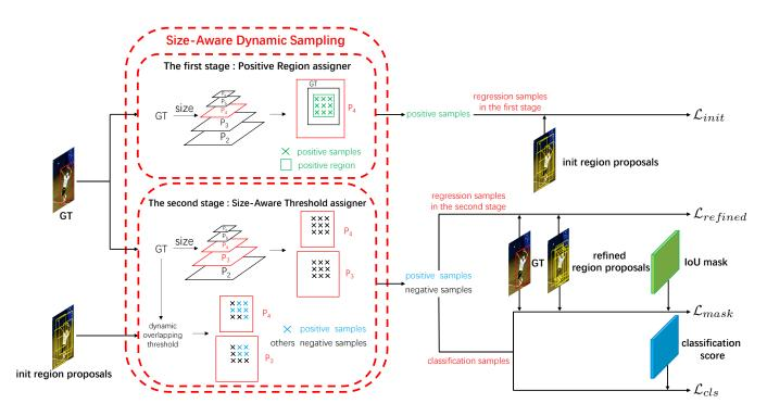
Fig. 2. The training phase of SC-RPN with Size-Aware Dynamic Sampling (SADS). In the first stage, positive samples are output and all of them are regarded as regression samples. Then in the second stage, positive and negative samples are output, among which all the positive samples are regarded as regression samples, while all the positive samples and the negative samples after random sampling are regarded as classification samples.
