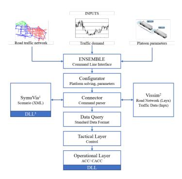
Figure 1. Proposed cross-platform framework to emulate truck platoons in connection with traffic simulators
