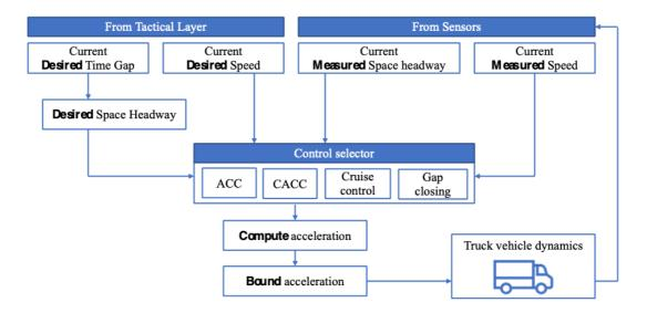
Figure 3. Operational layer framework
