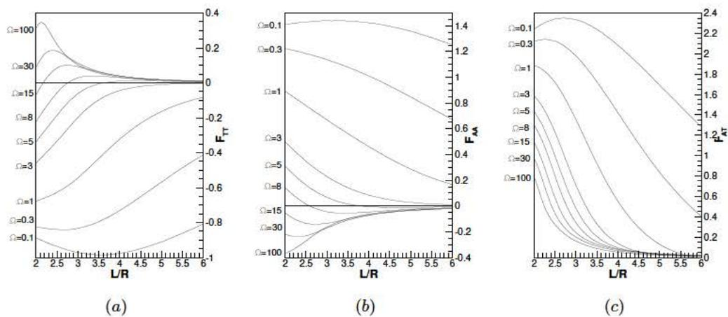
FIGURE 6. Forces exerted on the spheres due to steady streaming flow as function of the distance  $L/R$  for various values of  $\Omega$ : (a) axial force in transverse oscillation  $F_{TT}$ , (b) axial force in axial oscillation  $F_{AA}$ , (c) transverse force in oblique oscillation  $F_{AT}$ .
