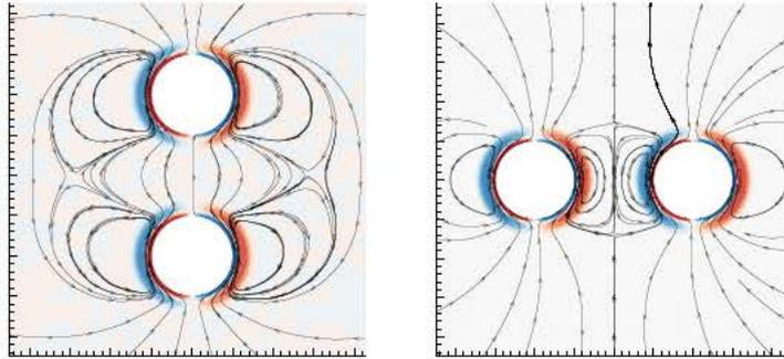
FIGURE 2. Oscillating flow around two spheres for  $\Omega = 100$ : (a) axial configuration, (b) lateral configuration. Streamlines and vorticity levels of the imaginary part.
