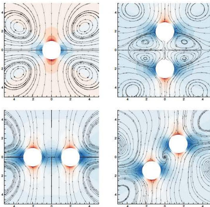
FIGURE 5. Steady streaming flow around one or two spheres for  $\Omega = 1$ : (a) Single sphere, (b) two spheres in axial configuration, (c) two spheres in lateral configuration, (d) two spheres in oblique configuration. ( $L/R = 4$  in (b, c, d))
