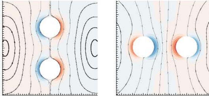
FIGURE 4. Oscillating flow around two spheres for  $\Omega = 1$ : (a) axial configuration, (b) lateral configuration. Streamlines and vorticity levels of the imaginary part.
