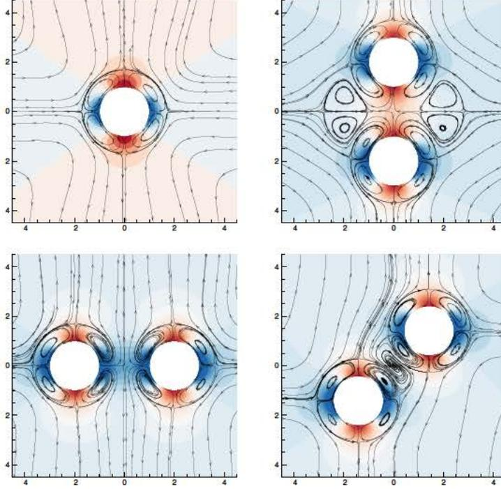
FIGURE 3. Streamlines and pressure contours of the steady streaming flow around one or two spheres for  $\Omega = 100$ : (a) Single sphere, (b) two spheres in axial configuration, (c) two spheres in lateral configuration, (d) two spheres in oblique configuration. ( $L/R = 4$  in (b, c, d))
