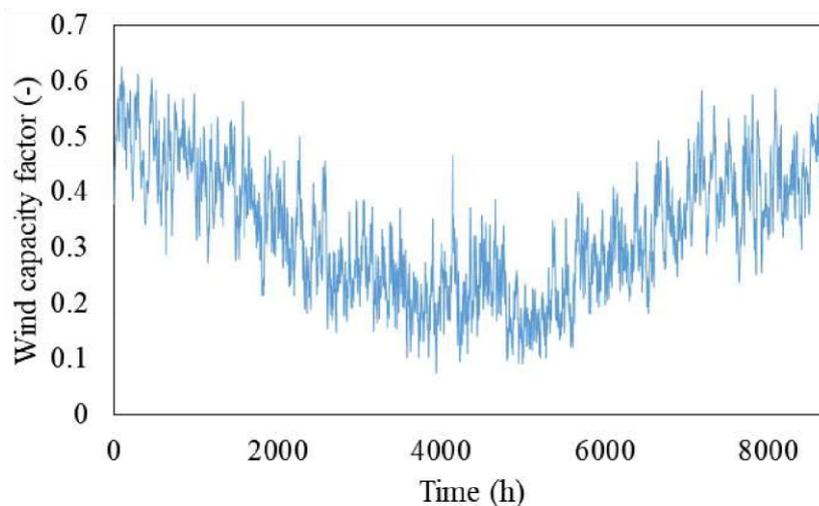
Fig. 3. Yearly wind capacity factor for a typical Belgian location.
