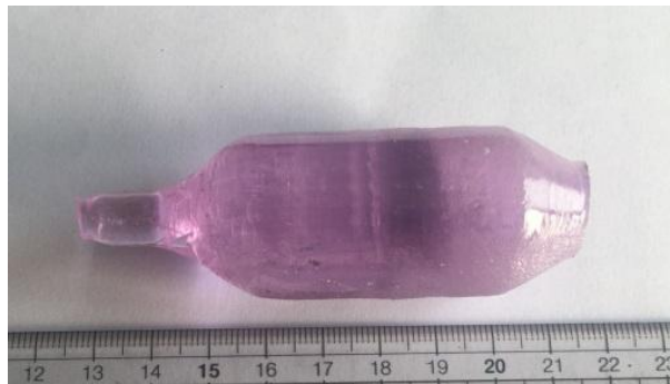
Fig. 1. As-grown single crystal ingot of Nd:SRA.
