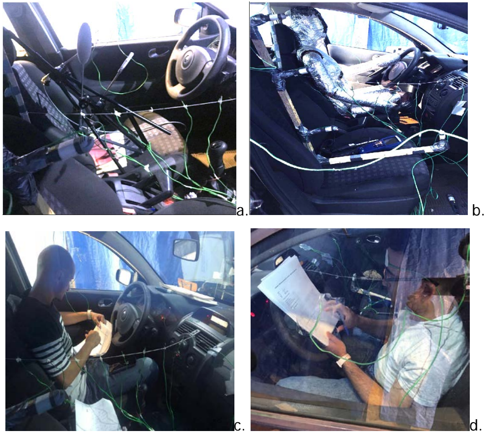
Fig. 6. Photographs from the experimental campaign: a) Comfort Sense measurements, b) Thermal manikin measurements, c, d) Human subjects measurements
