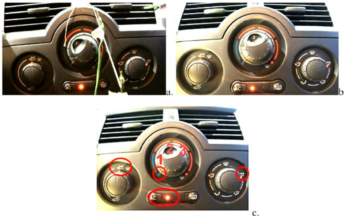
Fig. 5. Setup of the three position of the ventilation/cooling system a) V1, b) V2, c) V3
