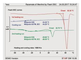
Figure 2 Heating-cooling-heating measurement of the racemate of menthol at 1000 K/s. For details, see text).
