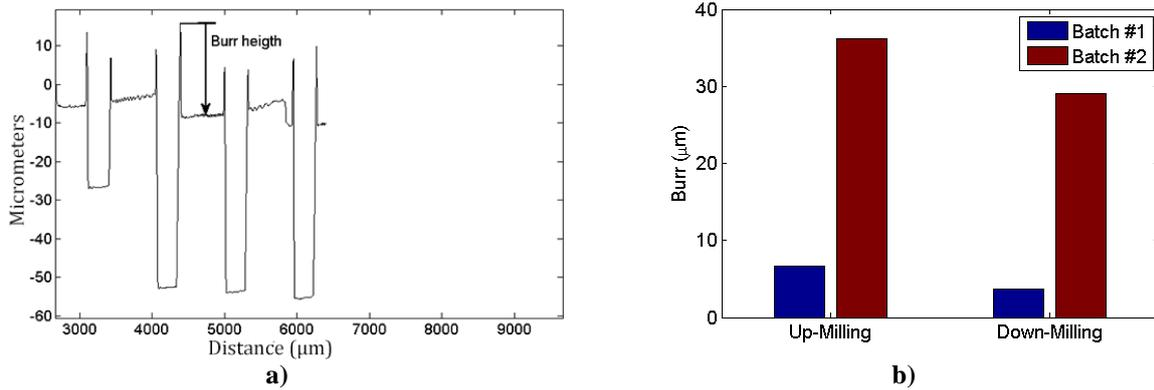
**Figure 3 – Analysis of burr formation: a) Measurement of top burr height; b) Comparison between burr height for batch #1 (feed of 2.5  $\mu\text{m}/\text{tooth}$  and depth of cut of 50  $\mu\text{m}$ ) and batch #2 (feed of 2.5  $\mu\text{m}/\text{tooth}$  and depth of cut of 40  $\mu\text{m}$ ).**
