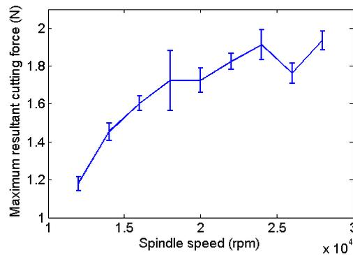
**Figure 8 – Cutting force evolution when increasing cutting speed.**
