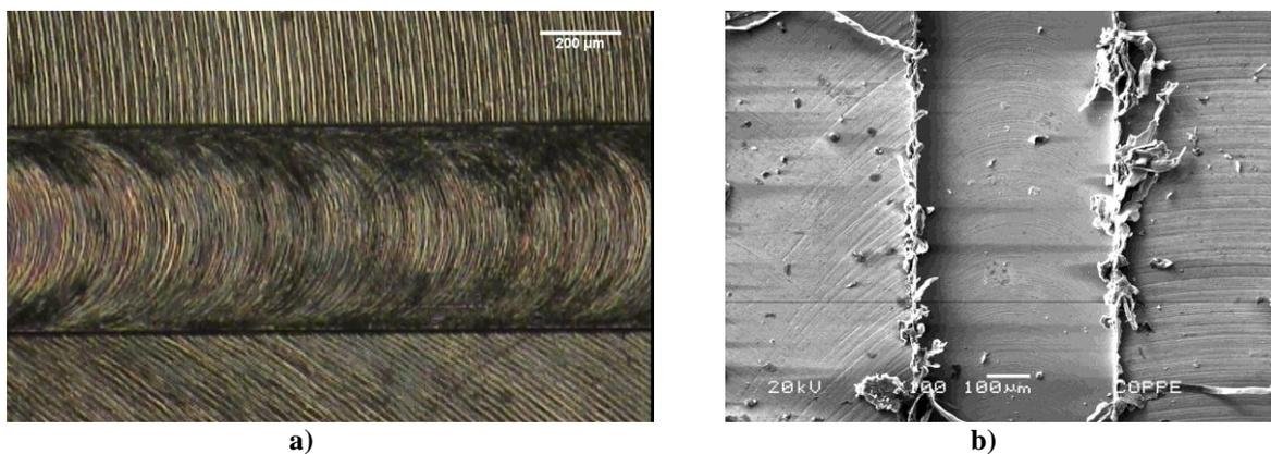
**Figure 2 – Scanning electron microscope images of the grooves: a) Batch #1, feed of 2.5  $\mu\text{m}/\text{tooth}$  and depth of cut of 50  $\mu\text{m}$  ; b) Batch #2, feed of 2.5  $\mu\text{m}/\text{tooth}$  and depth of cut of 40  $\mu\text{m}$ .**
