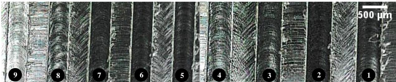
**Figure 4 – Machined slots image taken with a Handheld Digital Microscope (slots width: 500  $\mu\text{m}$ ).**
