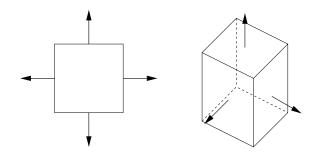
Figure 14.4: Degrees of freedom of the lowest-order Cartesian Raviart–Thomas element  $\mathbb{RT}_{0,d}^{\square}$  in dimensions two (left) and three (right, only visible dofs are shown).
