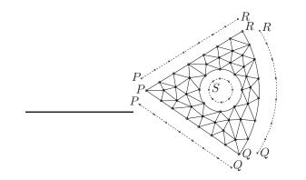
Figure 8.7: Meshing a two-dimensional domain.
