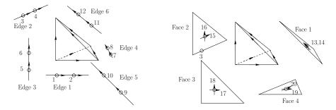
Figure 21.4: Enumeration of dofs for the  $\mathbb{N}_{2,3}$  element. Left: edge dofs. Right: face dofs.
