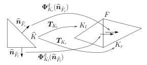
Figure 10.1: Orientation transfer for face normals.
