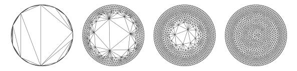
Figure 8.8: Triangulation of a circle by an advancing front method. Various stages of the mesh generation process are illustrated.
